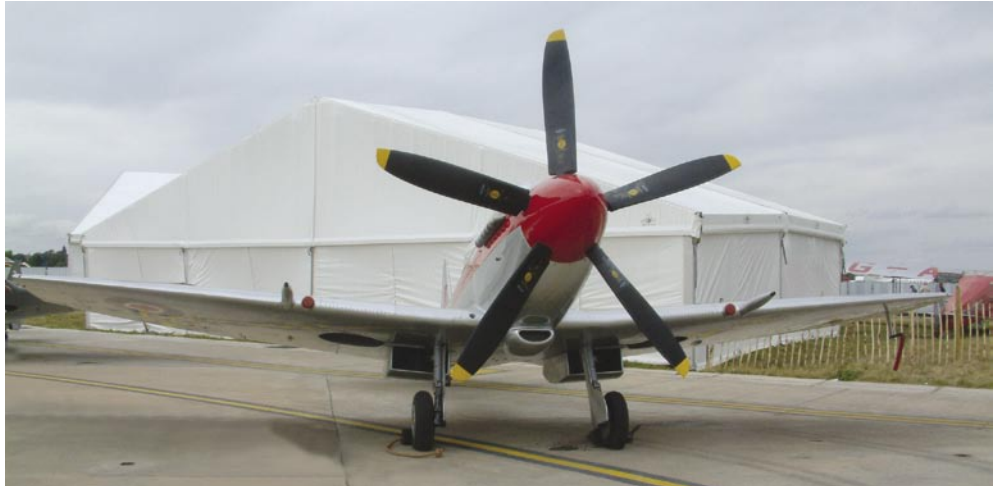
Figure 9.10b An increase in the number of blades will increase propeller solidity.
