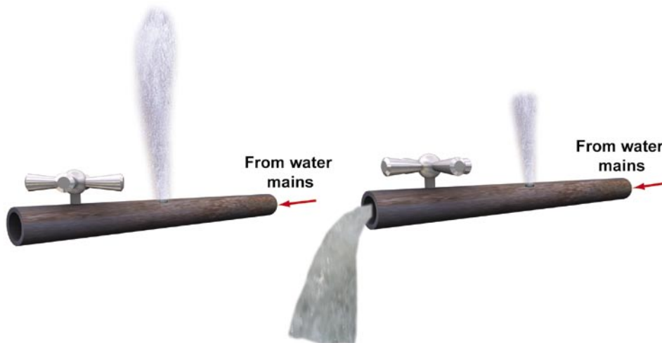
Figure 3.10 Bernoulli's Principle: The total energy of an ideal fluid is constant.
