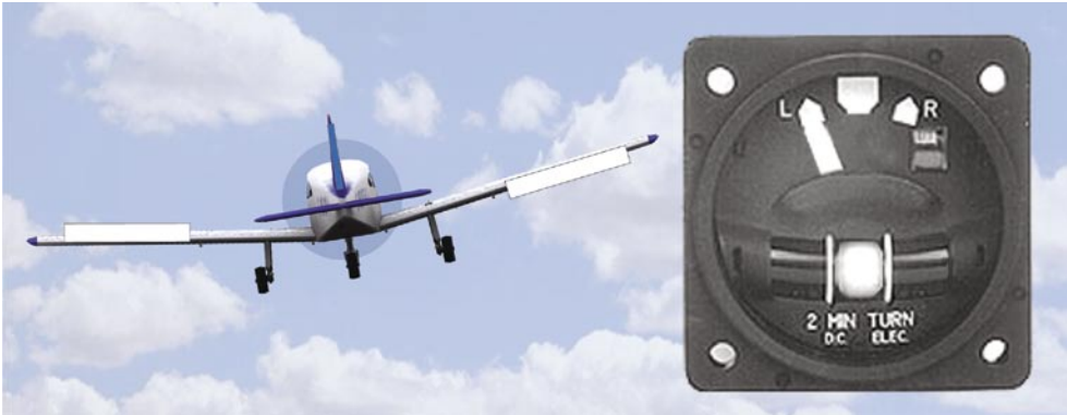
Figure 12.11 Adverse yaw has been eliminated. Here the aircraft is rolling to the left without adverse yaw. The ball's position "in the middle" shows that the aircraft is in balance.
