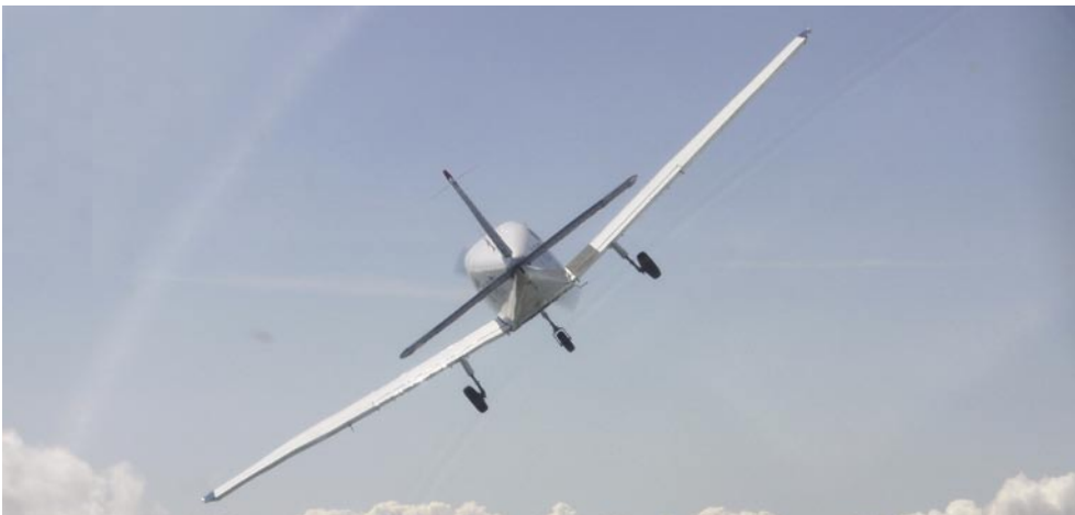
Figure 12.12 A PA28 established in a turn to the left, with the ailerons centralised.
